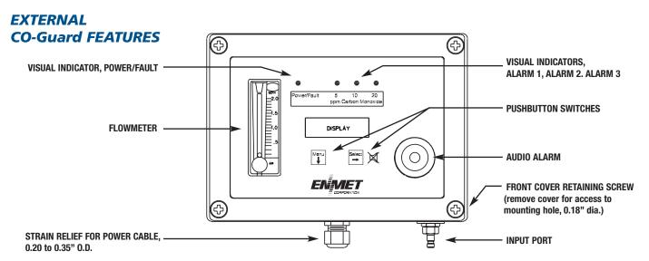
CO-Guard is supplied with a regulator and 5 foot hose for connection to the monitor. Connection from the facility air supply to the regulator is 1/4 inch NPT female.
